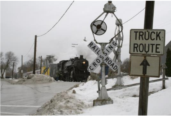
Wig Wag Signals in Plymouth, WI protect the movement of Soo Line #1003 in December 2008 during a Santa Train Movement. Photos by Dave Nelson
