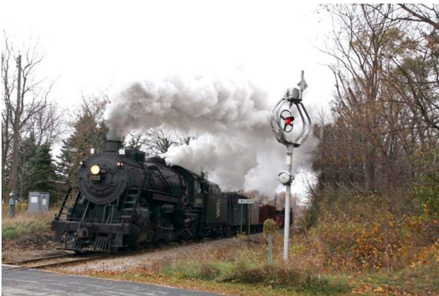
The Milwaukee Road had wig wag signals too. Here the Soo #1003 passes a wig wag that protects Lima Center Road in Lima Center, WI in November 2008. Photo by Keith Schmidt
